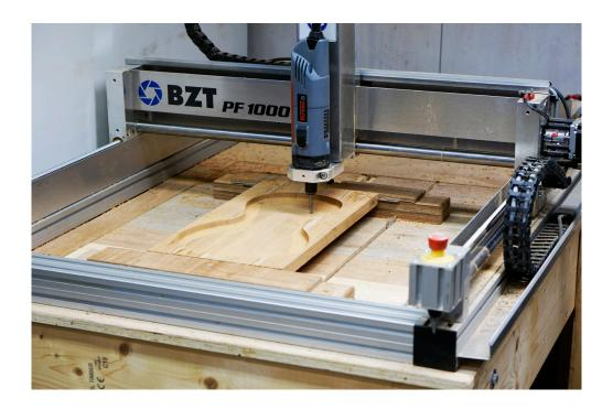
The zero point on the mill is 25 mm in front of the fixed center.
